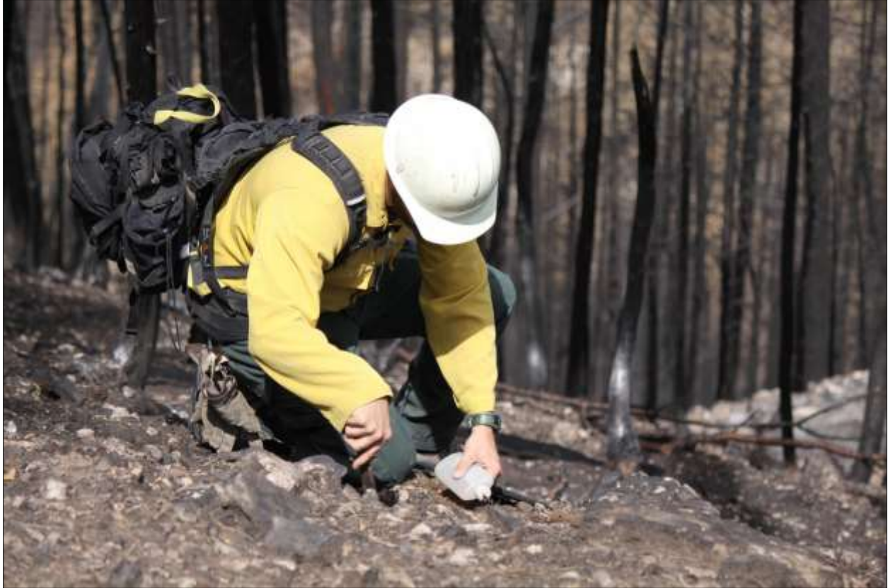
Micah Kiesow, soil scientist with the Kaibab National Forest and part of the Burned Area Emergency Response team on both the Stina Fire and Cat Fire, conducts a soil water repellency test to assess burn severity of soils and assess the viability of roots to help mitigate erosion from potential damaging rain events. 8-29-2018. IMG_9303. Credit the U.S. Forest Service, Southwestern Region, Kaibab National Forest.
