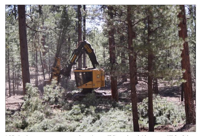
A feller-buncher operator removes green ponderosa pine up to 9" diameter breast height to create a 100-foot fuel break at pre-determined key locations specified by fire managers. In this instance, the fuel breaks will help give firefighters better "control lines" to stop a potential wildfire that could threaten the wildland-urban interface at Jacob Lake. Credit the USFS, Southwestern Region, Kaibab National Forest.
