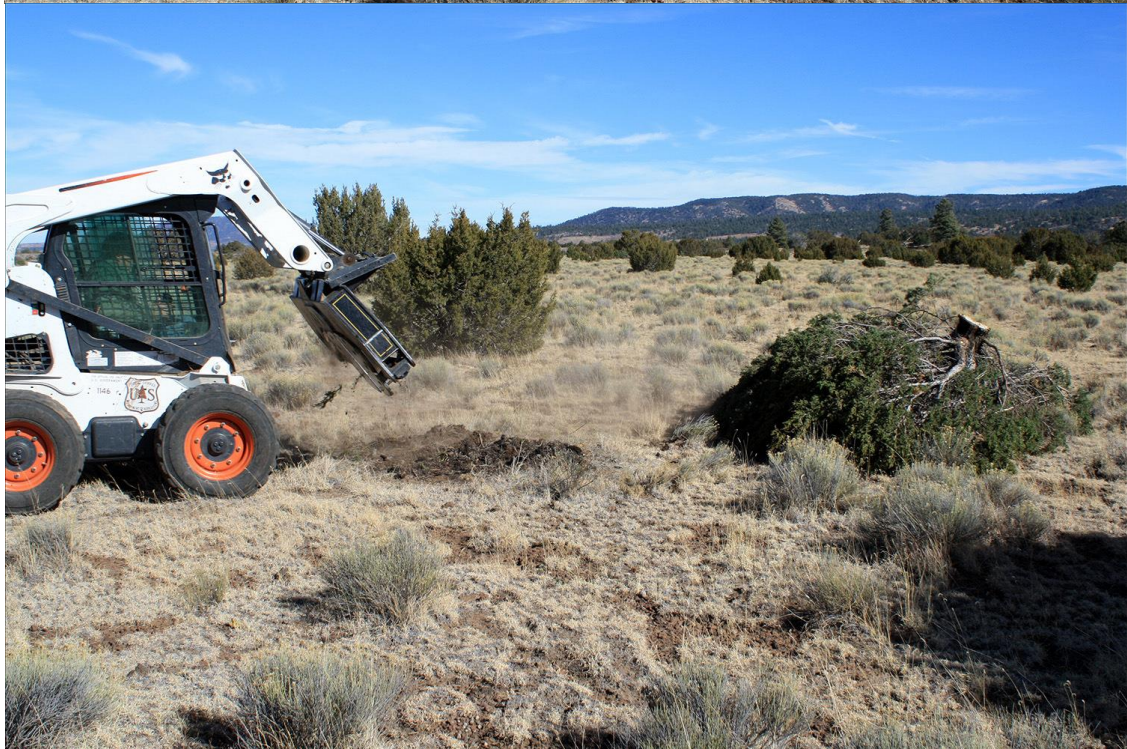
An agra-axe during and after removal of a conifer tree as part of grassland restoration.
