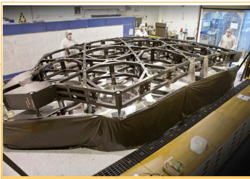
Figure 2: The center section of JWST's flight backplane structure following its completion at ATK.
